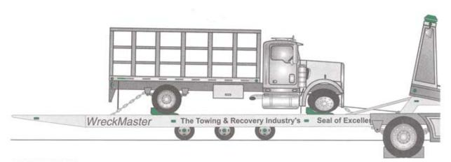
**CAUTION:** Install the SKATES before tilting the trailer's deck for unloading. Be sure the casualty or load is firmly secured to and controlled by, the winch line. If necessary, should you need to use any force to install a SKATE under a tire or load, use a short piece of 4 x 4 as a slide hammer at the back or heal of the SKATE when making contact. This should prevent any unnecessary damage to either the SKATE or to the casualty.
