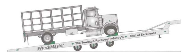
**CAUTION:** UNDER ANY CIRCUMSTANCES, *NEVER* allow any person or persons to be behind the trailer's deck while loading or unloading. ALWAYS be aware of the very dangerous area behind and surrounding your trailer. ONLY after the load has been completely secured on the trailer's deck should any person be allowed at the rear or behind the trailer's deck.
