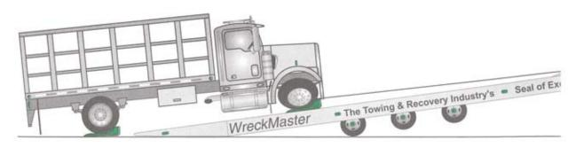
**CAUTION:** SKATES are intended for general use, such as loading and unloading from a trailer's deck or other platform. Do not attempt to move the casualty or load any farther than is absolutely necessary with your SKATES installed. SKATES may be subject to excessive wear when used on abrasive surfaces, such as asphalt, concrete and other extremely rough surfaces. SKATES are very versatile however and do have other limited use.
