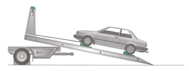
**CAUTION:** UNDER ANY CIRCUMSTANCES, *NEVER* allow any person or persons to be behind the carrier's deck while loading or unloading. ALWAYS be aware of the very dangerous area behind and surrounding your carrier. ONLY after the load has been completely secured on the carrier's deck should any person be allowed at the rear or behind the carrier's deck.
