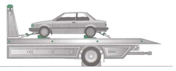
**CAUTION:** Install the SKATES before tilting the carrier's deck for unloading. Be sure the casualty or load is firmly secured to and controlled by, the winch line. If necessary, should you need to use any force to install a SKATE under a tire or load, use a short piece of 4 x 4 as a slide hammer at the back or heal of the SKATE when making contact. This should prevent any unnecessary damage to either the SKATE or to the casualty.
